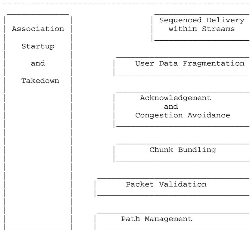
Figure 2: Functional View of the SCTP Transport Service
