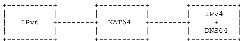
Figure 12: NAT64; DNS64 in IPv4-Only Hosts
