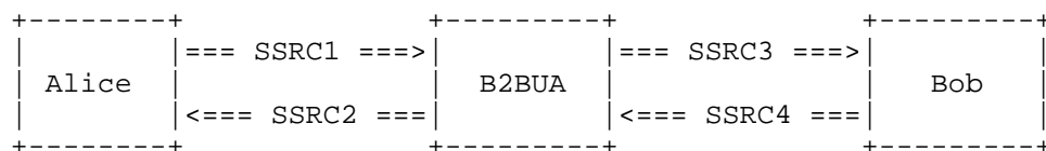
Figure 1: B2BUA Modifying RTP Headers
