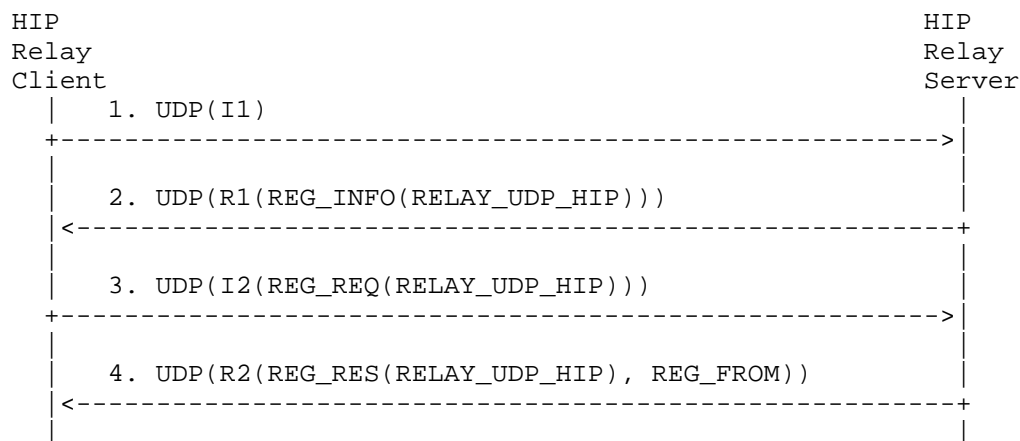
Figure 2: Example Registration with a HIP Relay
