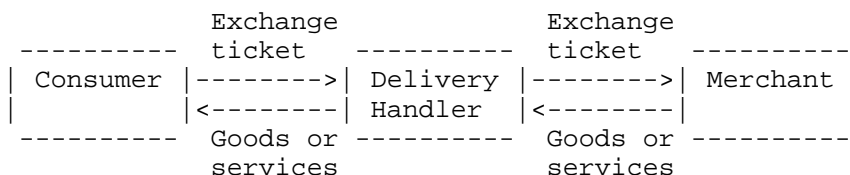
Figure 3. Coordination of untrusted participants using exchange ticket
