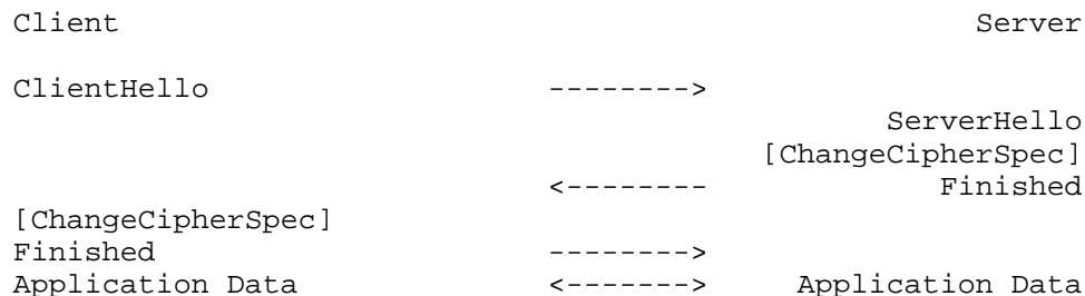
Fig. 2 - Message flow for an abbreviated handshake
