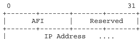
Figure 2: Interface Address Sub-Object
