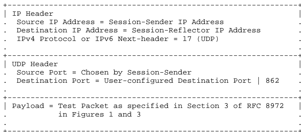
Figure 3: Content of Session-Sender Test Packet
