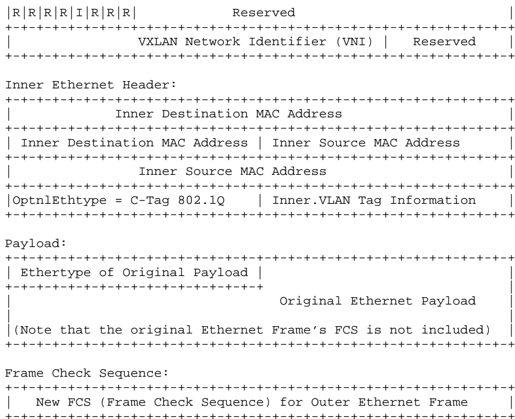
Figure 2: VXLAN Frame Format with IPv6 Outer Header
